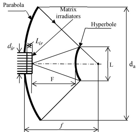
Fig. 2. Scheme of a two-mirror antenna
