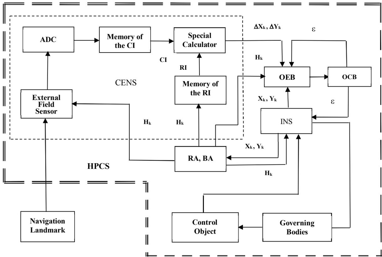
Fig. 1. Generalized structural diagram of a high-precision control system for high-speed aircrafts
