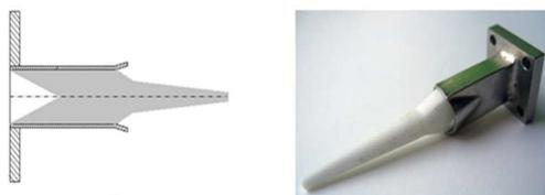
Fig. 4. Use of tapered dielectric rod in a multi-element antenna
