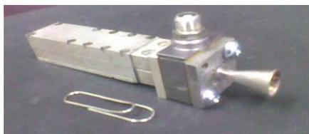
Fig. 5. Radiometric straight receiver gain 3 mm band
