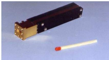
Fig. 3. Radiometric straight receiver gain 8 mm band
