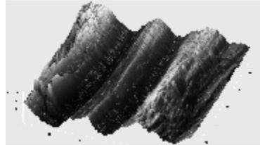
Fig. 12 – 3D image of worn surface for uncoated surface
