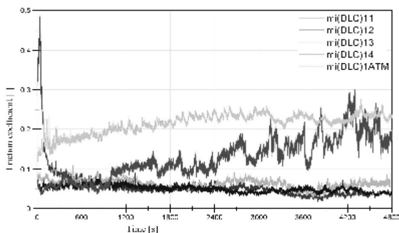
Fig. 8 – The coefficient of friction as a function of time for the friction pair DLC coated steel surface and WC ball
