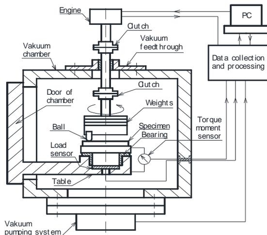
Fig. 2 – Schematic illustration of Vacuum tribometer device
