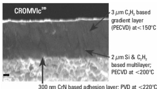
Fig. 4 – SEM view of DLC coating [3]
