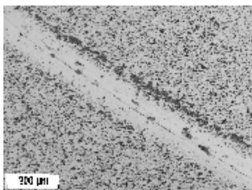
Fig. 9 – The microscopic image of worn surface for DLC coating CROMVIC2®
