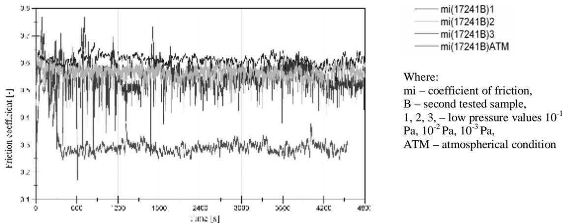
Fig. 6 – The coefficient of friction as a function of time for uncoated surface of disc (17241) and ball from bearing steel (14109)
