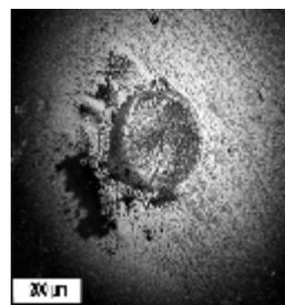
Fig. 10 – The microscopic image of worn surface for WC ball
