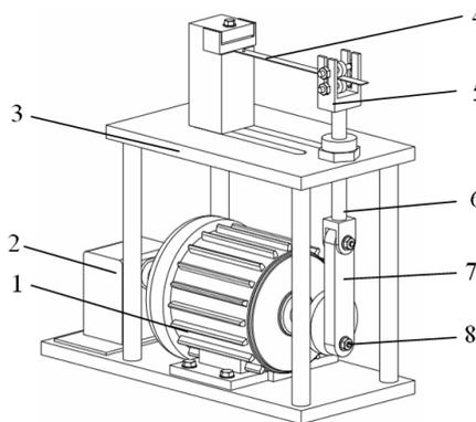
Fig. 1. Machine for the loading by cyclical cantilever bending: 1 – motor; 2 – cycles gage; 3 – element of the testing machine supporting frame; 4 – specimen for fatigue tests; 5 – movable grip of the testing machine; 6 – screw for the control of the stress ratio; 7 – rod; 8 – flywheel.
