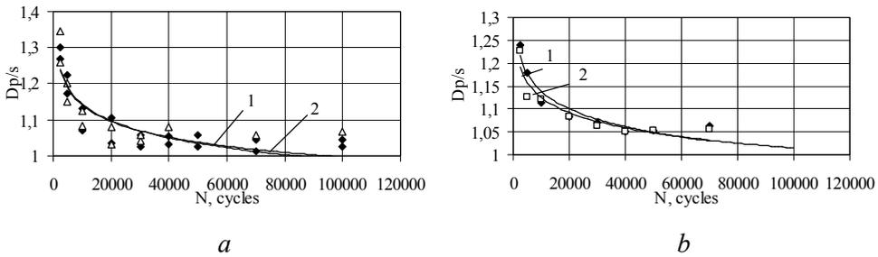
Fig.3. The change of fractal dimension  $Dp/s$  of deformation relief clusters at the maximum stresses of the cycle: 168 MPa (a) and 189 MPa (b): 1 – at the room temperature; 2 – at the blowing hot air temperature 60°C
