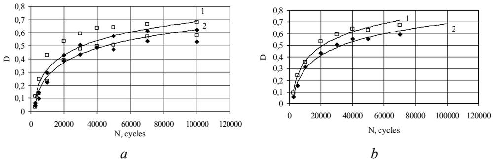
Fig.2. The evolution of the deformation relief saturation at the maximum stress of the cycle: 168 MPa (a) and 189 MPa (b): 1 – when the blowing hot air temperature  $60^{\circ}\text{C}$ , 2 – at room temperature
