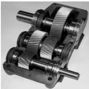
Fig. 5. Double-reduction gearbox with noncircular gears
