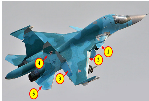
Fig. 2. SU-34 flight control surfaces scheme: 1 – two consoles canards; 2 – two sections rotary wing socks; 3 – two sections flaperons; 4 – two sections rudder; 5 – two consoles horizontal tail
