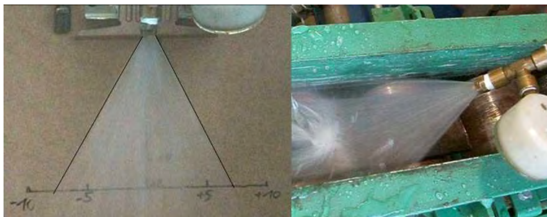
Figure 2.1 – Jet characteristic of one Lechler nozzle (left) and the water jet in the cooling line (right)
