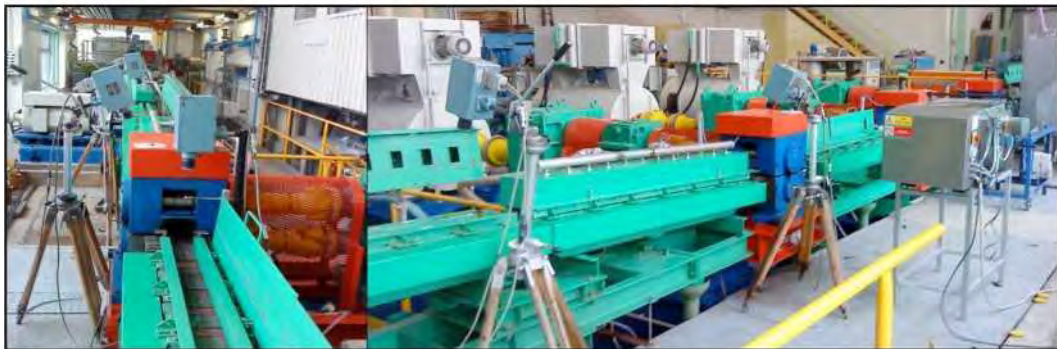
Figure 2.2 – Run-out table of laboratory plant (left: view in rolling direction; right: furnace and cooling segment, rolling direction from right to left)
