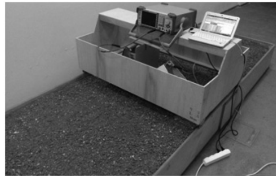
Fig. 1. Measurement set up with network analyzer
