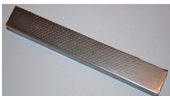
Fig. 2. Billet after hardness measurements on the device TP-5006 (Russia)
