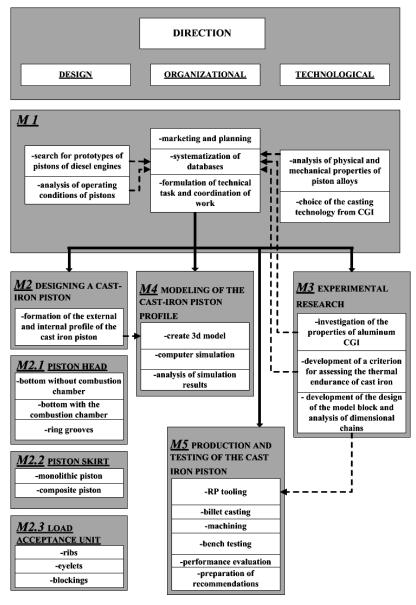
Fig. 1. System for organizing the modular design of cast-iron pistons for internal combustion engines
