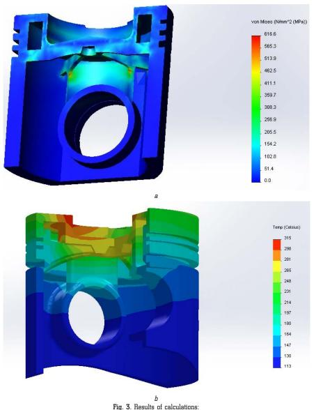
a – stress-strain state (0–616.6 MPa); b – temperature distribution in the piston (113–315 °C)
