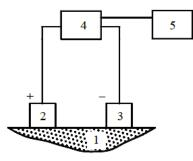
Fig. 3. The scheme of the hardware-software diagnostic complex «Intera-DiaCor» (Ukraine): 1 – human skin; 2 – «active» electrode; 3 – «passive» electrode; 4 – device for electropuncture diagnostics; 5 – personal computer
