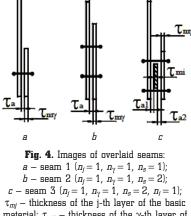
material;  $\tau_{m\gamma}$  – thickness of the  $\gamma$ -th layer of the lining;  $\tau_{\text{mi}}$  – thickness of the i-th layer of the plate;  $\tau_{a1}$  and  $\tau_{a2}$  – respectively, the thickness of the 1st and 2nd air layer
