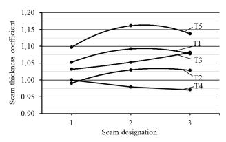
Fig. 8. Change in the seam thickness coefficient for seams: 1 - seam 1; 2 - seam 2; 3 - seam 3
