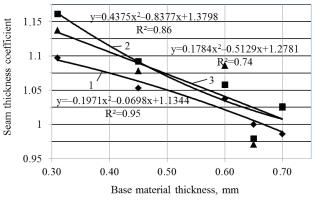
Fig. 7. Dependence of the seam thickness coefficient on the base material thickness: 1 - seam 1; 2 - seam 2; 3 - seam 3
