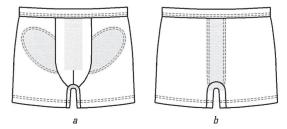
**Fig. 10.** Appearance of men's medical and preventive underpants: *a* – front view; *b* – back view. **Note:** gray color indicates the location of the overlays with silver plates
