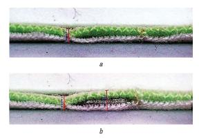
**Fig. 6.** Photographs of overlaid seams in a section (material T4): *a* – without a silver plate (seam 2); *b* – with a silver plate (seam 3)
