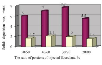
Floccules sedimentation rate after reagent injection, mm/s
