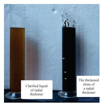
Fig. 2. Samples of clarified water and thickened slime of a radial thickener
