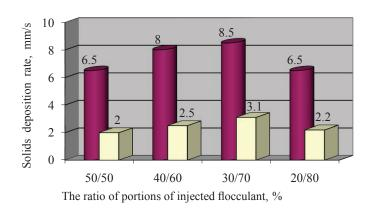
Floccules sedimentation rate after reagent injection, mm/s
