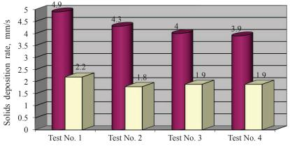
Floccules sedimentation rate after reagent injection, mm/s
