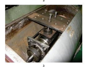
Fig. 5. Technological equipment for vibration-centrifugal reinforcement of the internal surfaces of cylindrical products on the vibrator of volumetric processing: a – technological equipment with bushing assembly; b – technological equipment in vibration machine with bushing assembly
