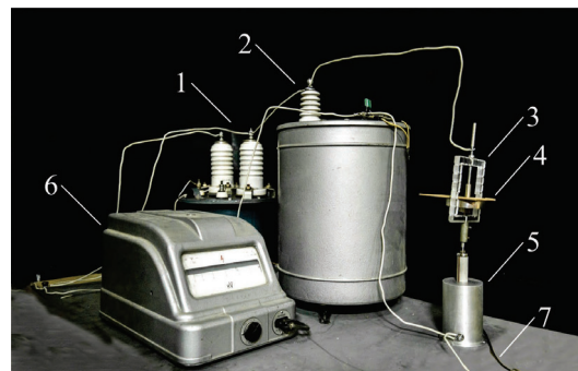
Fig. 1. Photograph of the experimental test stand for measuring the characteristics of partial discharges: 1 – step-up transformer; 2 – coupling capacitor; 3 – test object; 4 – electrical insulation cardboard (an element of the test object); 5 – shield of the high-pass filter; 6 – kilovoltmeter; 7 – cable for connection to an amplifier and an oscilloscope
