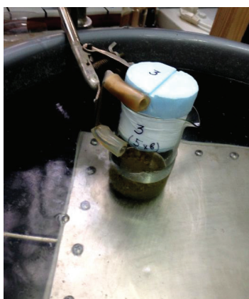
Fig. 1. Glass fixation in the stand of the ultrasound installation
