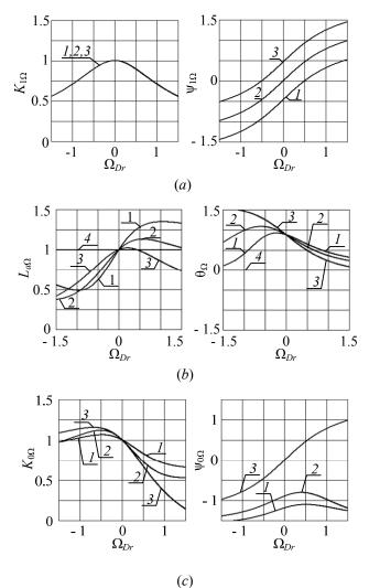
Fig. 2. Diagrams of normalized coefficients of the frequency functions  $K_{1\Omega}$  (*a*),  $L_{a\Omega}$  (*b*),  $K_{0\Omega}$  (*c*) and phase shift angles  $\psi_{1\Omega}$  (*a*),  $\theta_{\Omega}$  (*b*),  $\psi_{0\Omega}$  (*c*).
