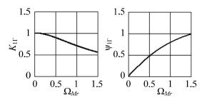
Fig. 4. Graphs of frequency responses of normalized transfer functions of amplitude modulation  $K_{1\Gamma}$  and its angles of the phase shift  $\psi_{1\Gamma}$ .
