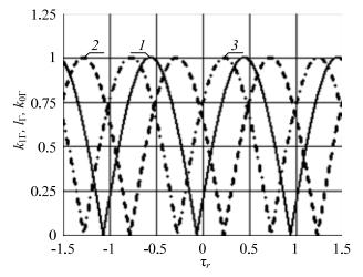
Fig. 3. Graphs of normalized amplitudes of modulation signals of the amplitude  $k_{1\Gamma}$  (curve *I*), the frequency  $l_{\Gamma}$  (curve 2) and auto-detection signal  $k_{0\Gamma}$  (curve 3) versus the normalized phase  $\tau_r = \delta_0/2\pi$  of the reflection factor.
