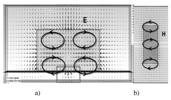
Fig. 7. Distribution of electro (a) and magnetic (b) fields of right adjacent parasitic mode at frequency of 7.13 GHz
