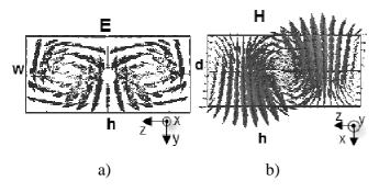
Fig.3. Distribution of electro (a) and magnetic (b) fields of  $TE_{21\delta}$  at frequency of 5.58 GHz
