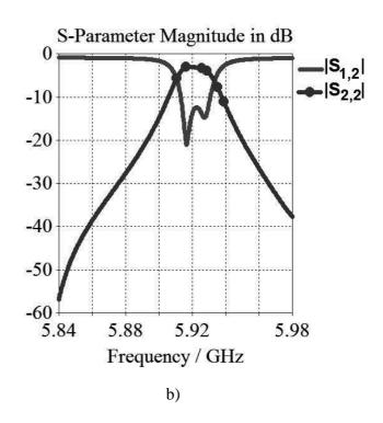
Fig. 11. S-parameters of the band-pass filter with "quadrupole" oscillation mode of DRs
