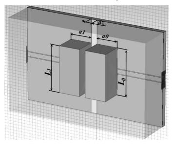
Fig. 10. 3D view of the band-pass filter with "quadrupole" oscillation mode of DRs
