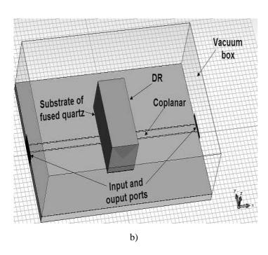
Fig.4. The dimensions (a) and general view (b) of the simulated DR with the  $TE_{21\delta}$  oscillation mode in a shielded coplanar transmission line
