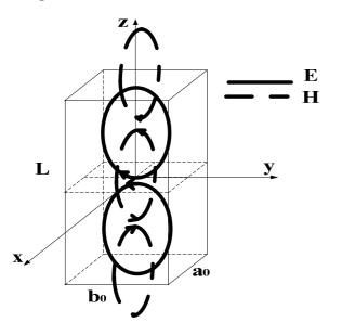
Fig.1. Distribution of electro-magnetic field of  $TE_{21\delta}$  oscillation mode
