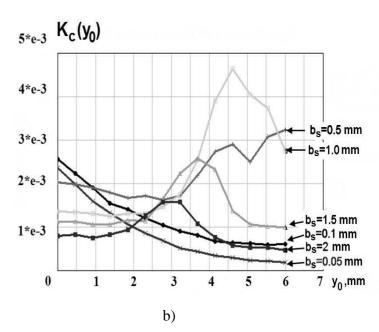
Fig. 9. Coupling coefficients of DR with the coplanar transmission line as a function of substrate's height bs (a) and displacement from the centerline  $y_0$  (b)
