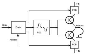
Fig. 3. Transmitter functional diagram.
