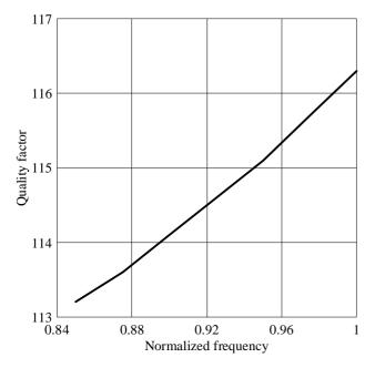
Fig. 6. Loaded quality factor of the resonator with correcting elements versus the normalized frequency.
