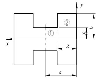
Fig. 3. Double ridged waveguide cross-section and coordinate system for the entire resonator configuration.
