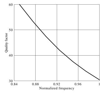
Fig. 7. Loaded quality factor of the resonator without correcting elements versus the normalized frequency.
