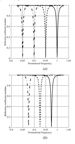
Fig. 4. Responses of the reflection coefficient modulus of the resonator with the correcting capacitive elements versus the normalized frequency under tuning the resonator on the variety of resonance frequencies.
