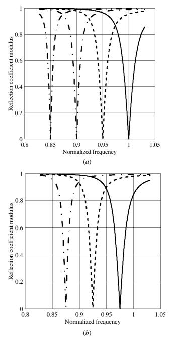
Fig. 5. Characteristics of the tunable resonator without the correcting capacitive elements on the variety of resonance frequencies.
