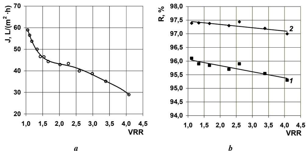
**Fig. 4. Permeate flux  $J$  (a) and retention  $R$  (b) of NanoRO membrane during the concentration of nanofiltration whey permeate ( $\Delta P=3.0$  MPa):**
