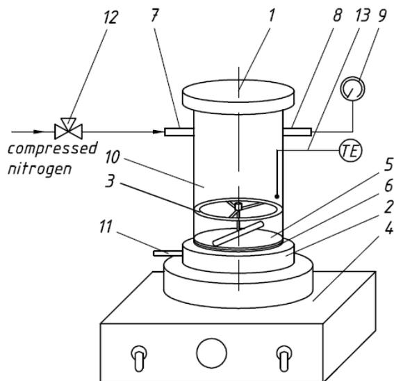
**Fig. 1. Schematic diagram of the dead-end laboratory setup:**
