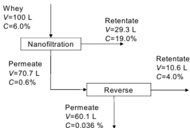
**Fig. 5. Material flows on the process flow diagram of two-stage whey treatment by nanofiltration and reverse osmosis:**
