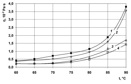
Figure 2. Changes of the effective viscosity of wheat starch suspensions depending on the treatment temperature at the concentration of Tween 20 (E432):  $I = -0; 2\Diamond - 0.1; 3\Delta - 0.2; 4\Box - 0.3$
