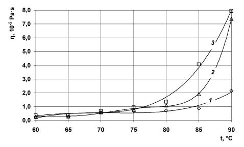
Figure 5. Changes of the effective viscosity of "Wheat starch – Tween 20 (E432) – white sugar" model systems depending on the treatment temperature at the concentration of citric acid, %:  $I\Diamond - 0; 2\Delta - 0.5; 3\circ - 1.0$
