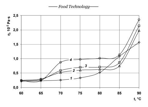
Figure 3. Changes of the effective viscosity of "Wheat starch – Tween 20 (E432)" model systems depending on the treatment temperature at the white sugar concentrations, %:  $I\diamond - 0; 2\Delta - 5.0; 3\Box - 10.0; 4\diamond - 20.0$
