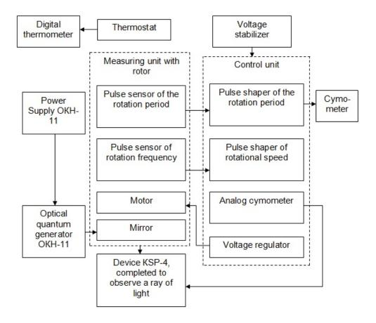
Figure 1. Electric structural scheme of viscometer VPN-0.2M
