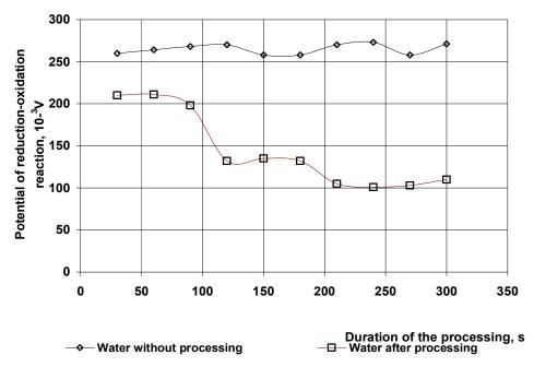
Figure 5. Investigation of the potential of reduction-oxidation reaction during the experimental water processing
