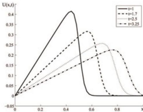
Fig. 10. Shock propagation,  $\lambda = 0.005$ .
