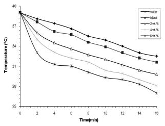
${\it Fig. 8.}$  Solidification curves of the (CMC-PVP-MgO) nanocomposite
