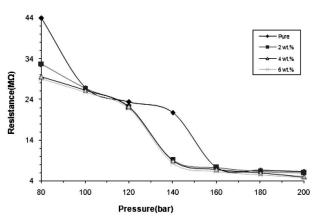
${\it Fig.~6.}$  Effect of the pressure on electrical resistance of the (CMC–PVP–MgO) nanocomposite for different concentrations of MgO nanoparticles
