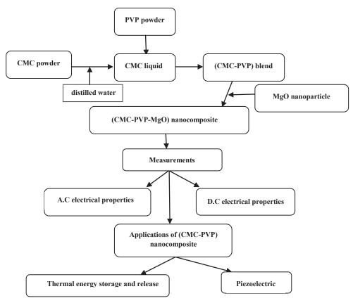
Fig. 1. Diagram of the experimental work
