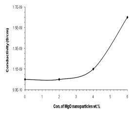
Fig. 5. Variation of the DC electrical conductivity of the (CMC–PVP) blend with the concentration of MgO nanoparticles
