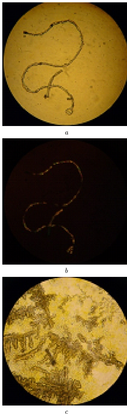
Fig. 8. Images of ( a and b ) a dye- 3 film obtained from the aqueous solution and ( c ) a hybrid film dye 3 -CdTe nanocrystals from the electrolyte solution. The magnification is \Gamma = 200 . Images ( a ) and ( c ) were obtained in non-polarized light and ( b ) in crossed polarizers
