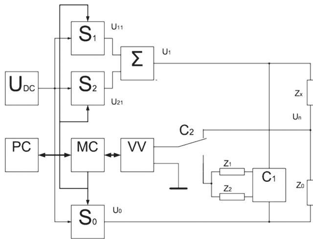
Fig. 2. High impedance bridge with phase controlled balance
