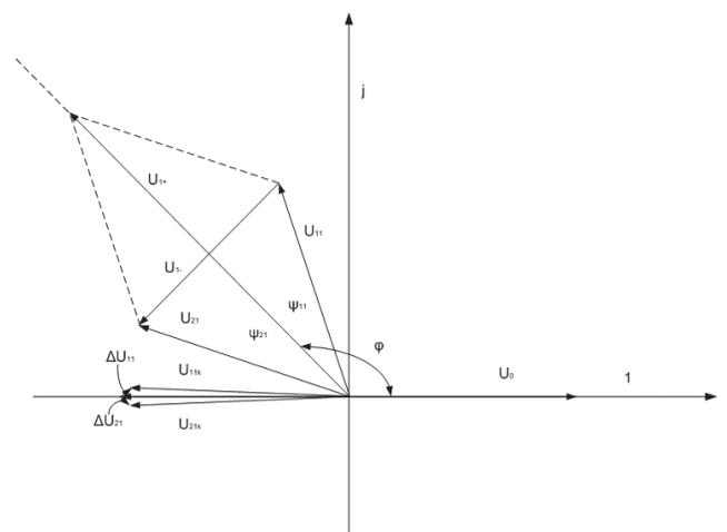
Fig. 1. Phase control vector diagram
