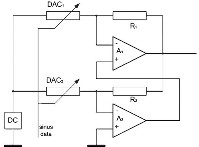
Fig. 6. Generator's iterative structure
