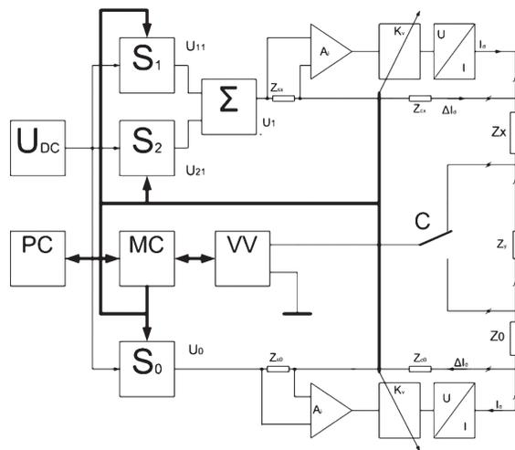
Fig. 3. Four terminal bridge diagram (without calibration divider)
