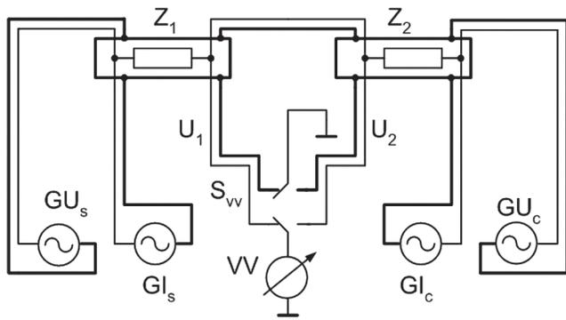
Fig. 4. Four pair terminal connection
