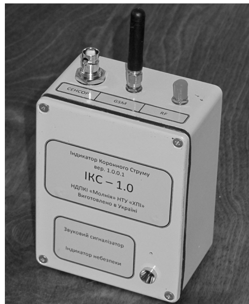
Fig. 3. The electronic devise of the field strength meter (X-1)
