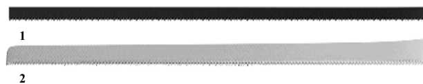
Fig. 6. Half section of the bunch density distribution at time of 0,6 ns(1) and 19 ns (2). v=2,7 \cdot 10^8 \text{ m/s} ( v/c=0,9 ), L=13,5\text{m}, n=5 \cdot 10^{12} \text{ m}^{-3}
