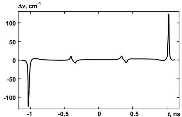
**Fig. 2. The instantaneous frequency shift of the laser pulse at the exit of a toluene-filled cell divided by the transparent partition**
