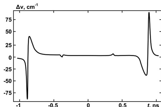
**Fig. 4. The instantaneous frequency shift of the laser pulse at the exit of a toluene-filled cell divided by the thin absorbing partition**
