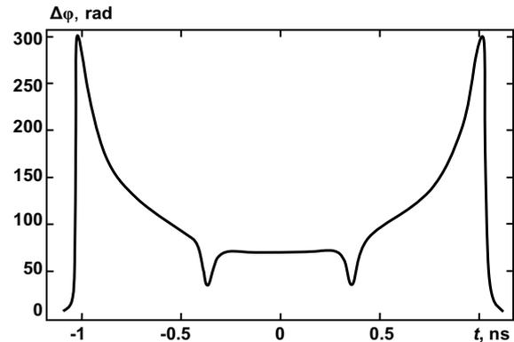
**Fig. 1. The self-induced phase shift of the laser pulse at the exit of a toluene-filled cell divided by the transparent partition**
