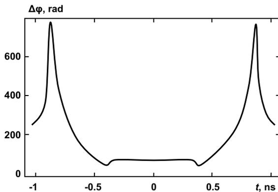
**Fig. 3. The self-induced phase shift of the laser pulse at the exit of a toluene-filled cell divided by the thin absorbing partition**
