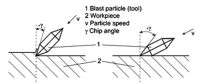
Fig. 3. Behaviour of a solid blasting abrasive at surface of a workpiece [3]
