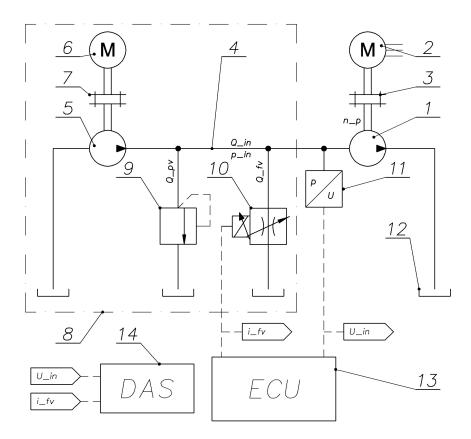
Fig. 2. Hydraulic system diagram of the test stand with the control system
