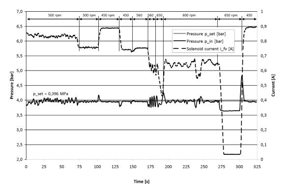
Fig. 6 Pressure changes in the inlet channel of the gear pump during the tests [8]
