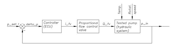
Fig. 3. Control system of the input pressure in the tested pump
