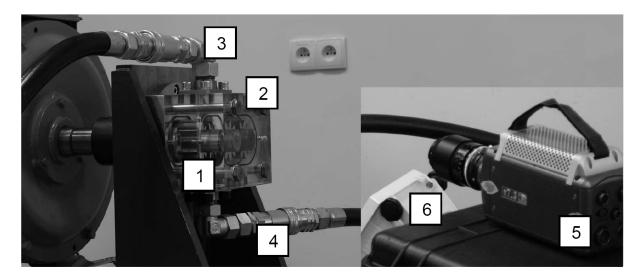
Fig. 1 Gear pump made of plastic at the test stand
