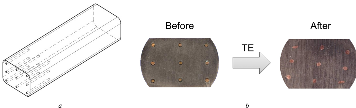
Fig. 4. Visualization of metal flow during TE: a) a sketch of the sample with embedded copper markers before TE; b) photographs of the sample cross sections with markers before and after TE
