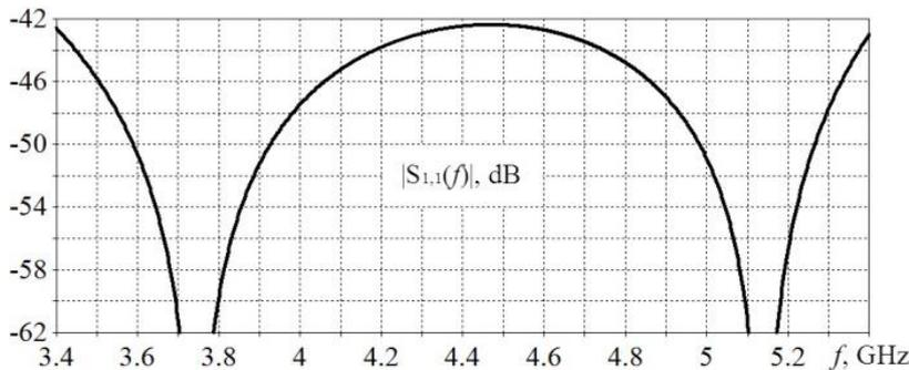
Fig. 6. The frequency dependence of minimized reflection coefficient of a right-angle coaxial junction
