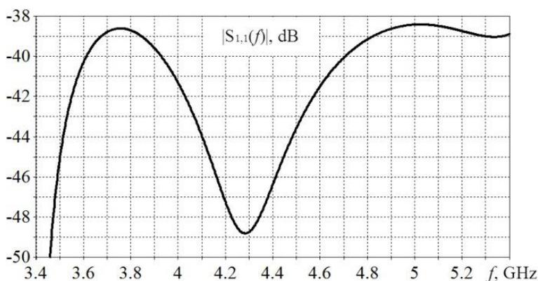
Fig. 8. The frequency dependence of minimized reflection coefficient of an antiphase power combiner/divider
