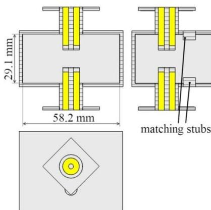
Fig. 7. The structure of an antiphase power combiner/divider
