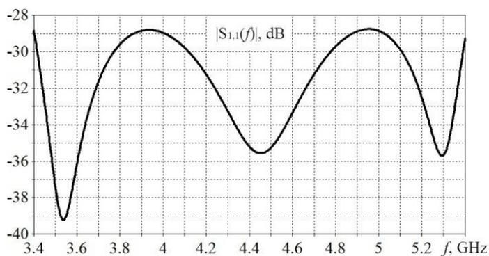
Fig. 4. Frequency dependence of the minimized reflection coefficient of the turnstile junction
