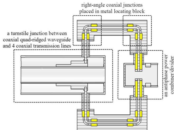
Fig. 2. Inner structure of the coaxial OMT
