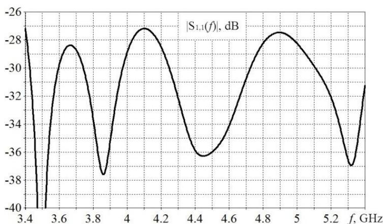
Fig. 9. The frequency dependence of minimized reflection coefficient of coaxial orthomode transducer
