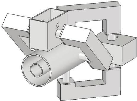
Fig. 1. General design of the coaxial OMT
