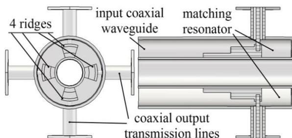
Fig. 3. The geometrical configuration of a turnstile junction
