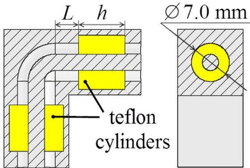
Fig. 5. The structure of a right-angle coaxial junction
