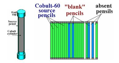
*Figs.2. (a) and (b). (a) Source pencil constructions. (b) Scheme of arrangement of sours pencils in the source module.*
