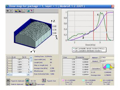
Fig.4. Left Graph: 3D view of the depth dose distributions of Gamma ray (Dose Map, along layer length (axis Y) and along layer width (axis X)) in graphical and tubular forms for the  $I^{st}$  layer in  $I^{st}$  package. The dose value is integrated along layer thickness (axis Z). Right graphs: Cumulative distribution function – cdf (curve 2), and Probability density function in I/kGy - pdf (curve 1).
