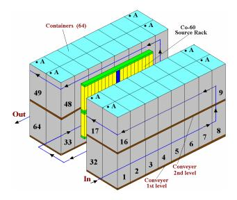
Fig.3. Sequence of irradiation in a flat panoramic  $Co^{60}$  source rack, multipass, two direction, multiposition. The 64 aluminum containers with product are moved around the  $Co^{60}$  source rack on a conveyor 8 passes at two levels. Point "A" is a fixed point on the side surface of the process load, which passes through the irradiation room on both sides of the  $Co^{60}$  source rack from position 1 to position 64.
