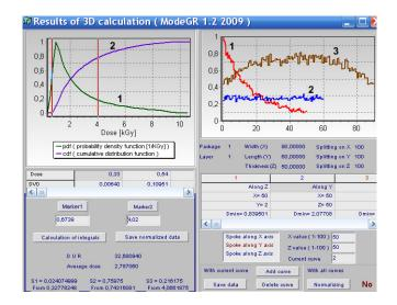
Fig.6. The form of "Results of 3D calculation" for analysis of 3D absorbed dose distribution of gamma rays for the 1<sup>st</sup> layer in 1<sup>st</sup> package. Left graphs-DVH analysis, Right graphs – spokes method analysis. 1<sup>st</sup> curve on the right graphs is the absorbed dose distribution along axis Z (layer thickness), 2<sup>nd</sup> curve - the absorbed dose distribution along axis Y, 3<sup>d</sup> curve - the absorbed dose distribution along axis X.
