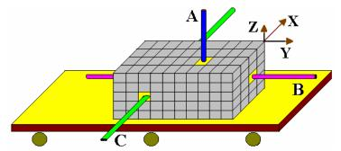
Fig.5. Target layer with grid and spokes located on a conveyer platform.
