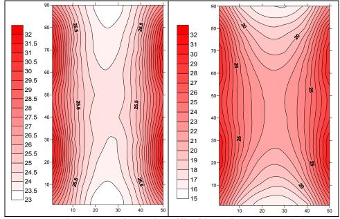
Fig. 5. Isodose curves in plane at the middle of the product container which is perpendicular to the source rack for 2 extreme cases. a) Metal density  $-0.001 \text{ g/cm}^3$ , DUR = 1.4, b) Metal density  $-7 \text{ g/cm}^3$ , DUR = 2.15
