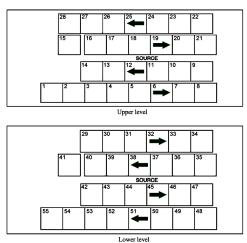
Fig. 2. The sequence of product totes movement at upper and lower levels
