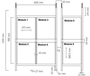
Fig.1. Arrangement of source modules in the NCRRT panoramic source rack with active cobalt-60 source pencils
