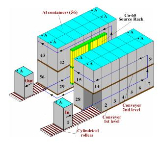
Fig.3. Sequence of irradiation in a flat panoramic Co<sup>60</sup> source rack, multi-pass, two direction, multi-position. "A" is a fixed point on the side surface of the process load, which passes through the irradiation room on both sides of the Co<sup>60</sup> source rack from position 1 to position 56, with four passes on each side of the source.
