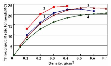
Fig.6. Curves 1 and 2 - dependence of product mass throughput at absorbed dose 1 kGy on product density for two irradiator designs by MDS Nordian, Canada. Curve 3 was calculated at density 0.002g/cm<sup>3</sup> of the metal layer, curve 4 - at density 1g/cm<sup>3</sup> of the metal layer
