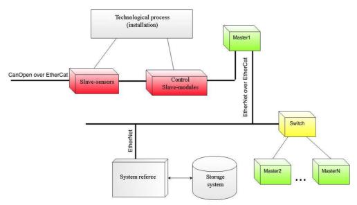
Fig.1. System with split-architecture management - PLC-technology
