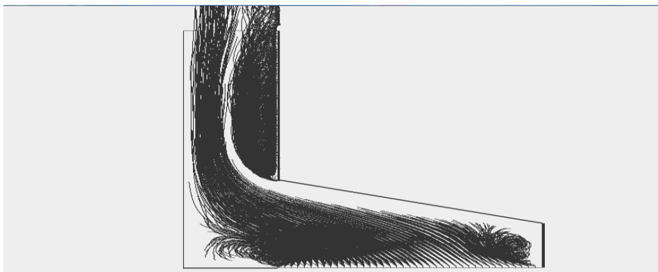
Fig.10 The gathering collector vorticity zone distribution when there are 1758 free vortices
