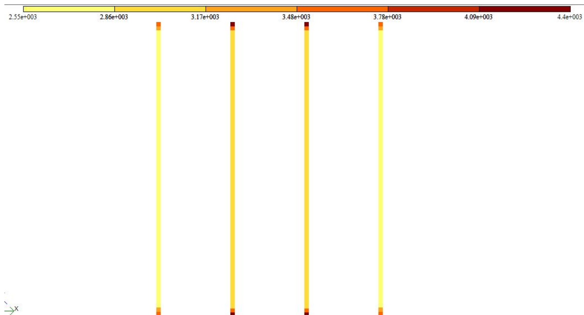
Fig. 3. Mosaics of distribution of the calculated base stiffness coefficient values under normal operating conditions
