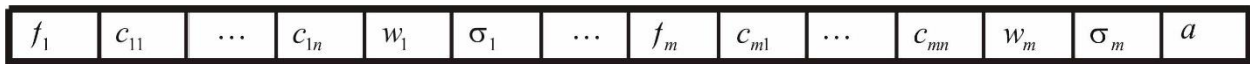
Fig. 2. Encoding configurable parameters RBF neural network in the form of antibodies (chromosomes)
