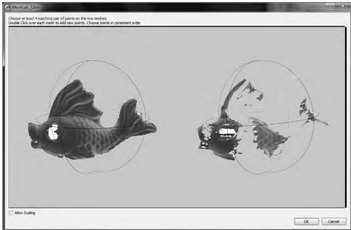
Fig. 3. Connection of scans on the junction points in Meshlab
