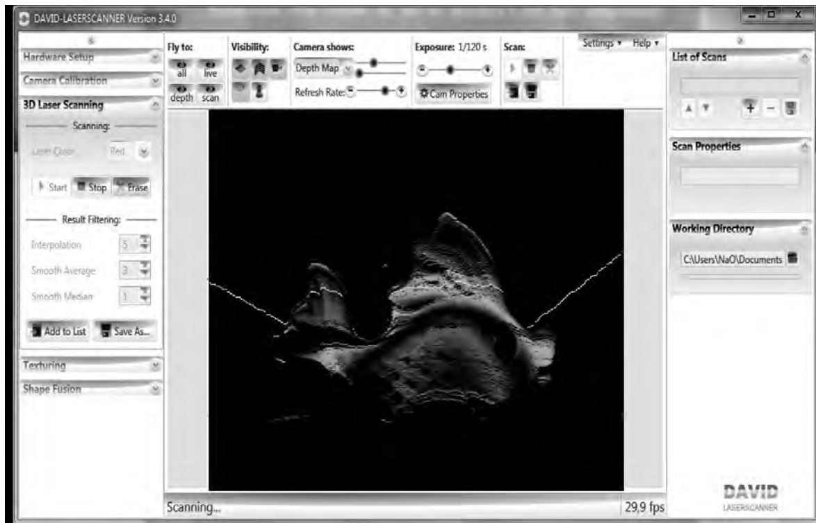
Fig. 2. The camera image while scanning mode maps depths
