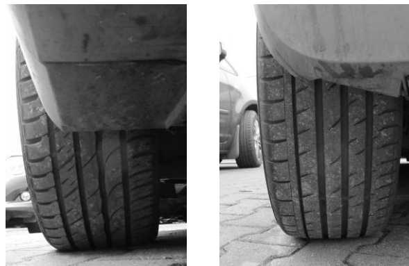
Fig.5 View of treads of tires used in road tests Barum BRAVURIS 2( on left) and Continental Conti Sport Contact 3( on right)
