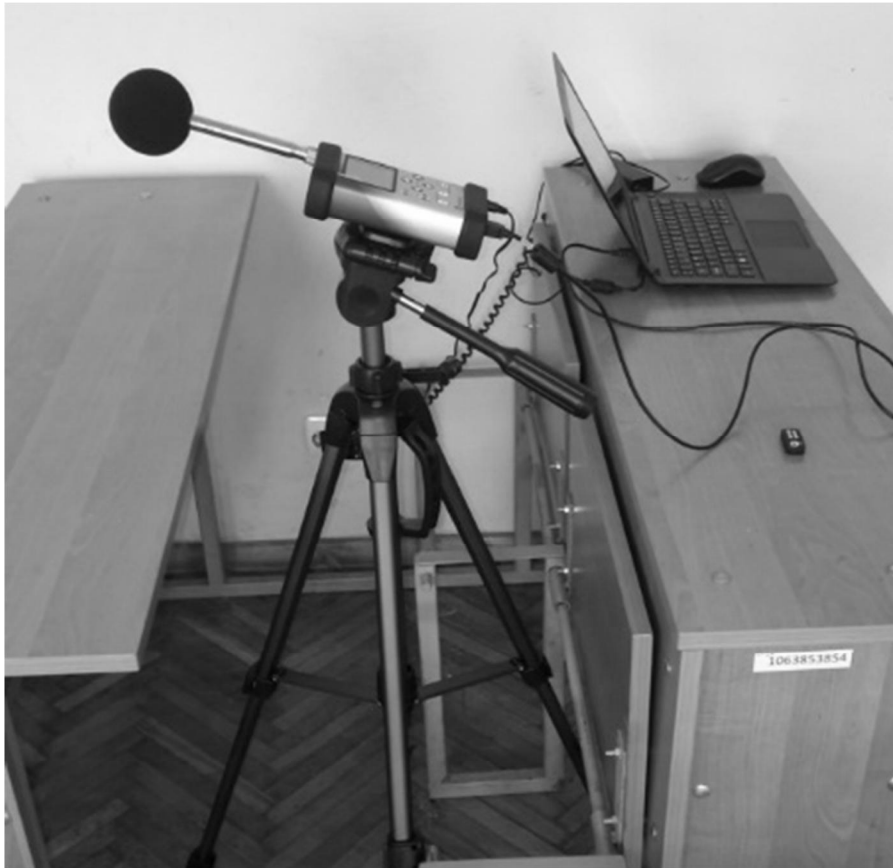
Fig. 2. Registration of the auditorium response to impulse noise source
