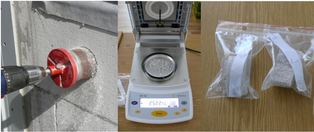
Fig. 1. Laboratory instruments for measurements of initial conditions – water profile
