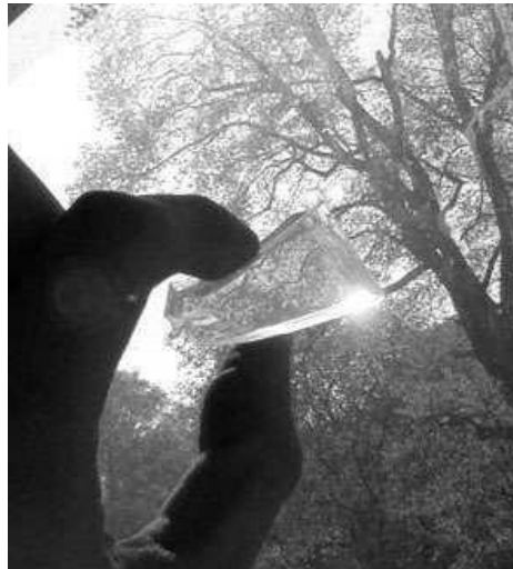
Fig. 9. Modern aerogel glass [8]
