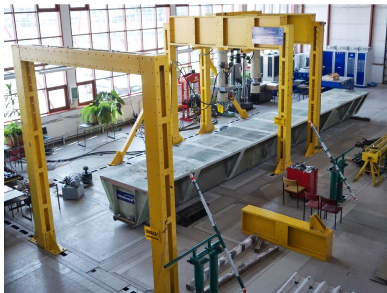
Fig. 11. The prototype girder at the testing stand in structural laboratory of RUT
