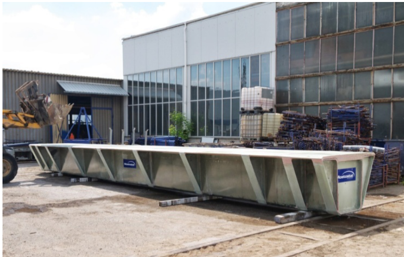
Fig. 7. The completed testing girder
