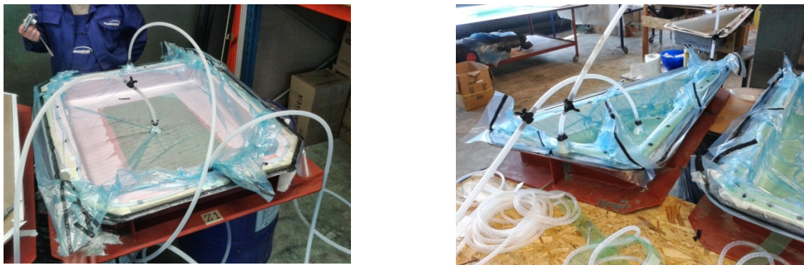
Fig. 5. Infusion process used for manufacturing of diaphragms and ribs (Mostostal workshop)
