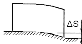
Fig. 4. Vertical dislocations of base under the foundations, which cause the difference of subsidence \Delta S of end walls in the facade plane
