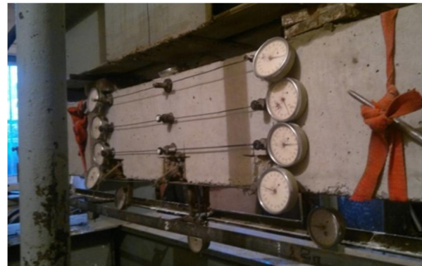
Fig. 7 The test beam. Placing instrumentation.
