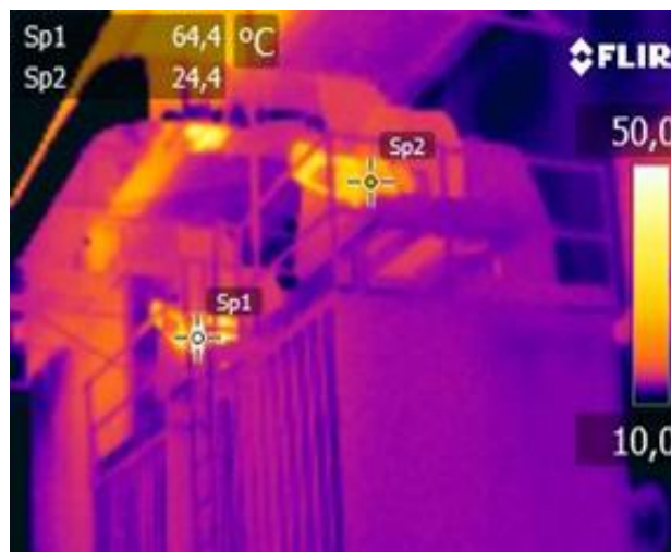
Fig. 1. Thermography of a ventilation system. The two electric motors are the same size and the same nominal load but the surface temperatures are very different: a warning sign of possible energy waste
