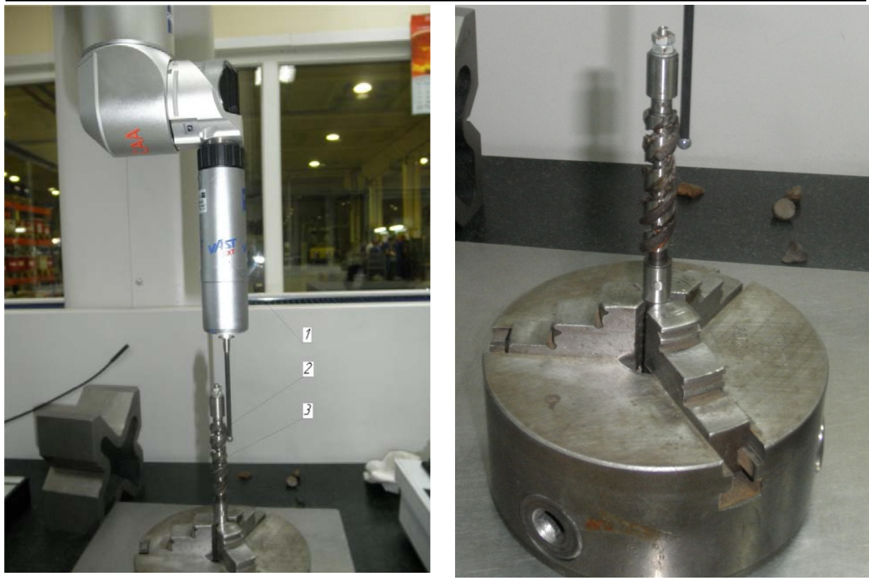
a) 1 – the reference machine Carl Zeiss CONTURA G2; 2 – sensor; 3 – HSH. a) general view of the measurement area of the external cylindrical contour of HSH; б) the measurement area of the external cylindrical contour of HSH; Fig. 5. Reference machine Carl Zeiss CONTURA
