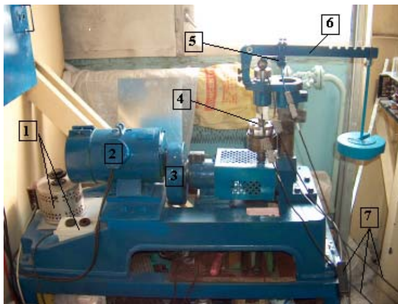
Fig. 1. General view of the modernized Amsler's machine: 1 – power and control; 2 – electric motor; 3 – planetary gear; 4 – head test of friction torque sensor; 5 – load force sensor; 6 – loading arrangement; 7 – connection to a capture measuring and recording system Source: Authors' own elaboration
