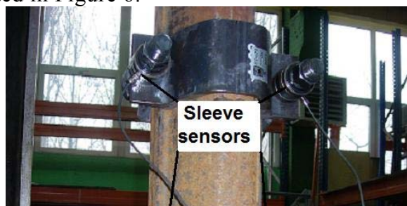
Fig. 6. View of frictional joint with assembled sleeve sensors on the bolts of stirrups
